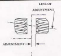
The Southern Style features the unique Automatic Helix Adjustment. The Helix path of the thread along the line of adjustment remains true and in alignment throughout the entire life of the gage.
