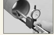
3. Rock the gage from side to side to locate the largest indicator reading.
