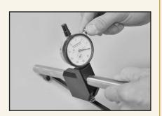
Place the contact point in the square notch of the setting standard.
