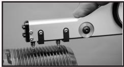
3. Apply pressure to the nose of the gage with the index finger. Do not apply excessive force to the gage, just enough to keep the moveable point in contact with the thread flanks. Then, using the rear contact point as the pivot point, sweep
