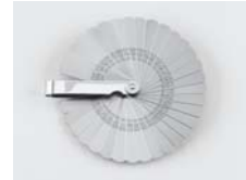
FG-35-3 $14.95 35 blades, 1/2" wide and 3" long. Thickness (in inches) .0015, .002, .003, .004, .005, .006, .007, .008, .009, .010, .011, .012, .013, .014, .015, .016, .017, .018, .019, .020, .021, .025, .026, .027, .028, .029, .030, .031, .032, .033, .034, .035
