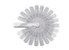
FG-22-STEP $29.65 22 blades, 1/2" wide and 3" long with .002 deep by 5/8" step ground at tip. Thickness (in inches) .004-.006, .005-.007, .006-.008, .007-.009, .008-.010, .009-.011, .010-.012, .011-.013, .012-.014, .013-.015, .014-.016, .015-.017, .016-.018, .017-.019, .018-.020, .019-.021, .020-.022, .021-.023, .022-.024, .023-.025, .024-.026, .025-.027
