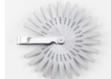
MFG-25-T-76 $30.00 25 blades, 12.7mm wide tapered to 6.35mm and 76mm long. Thickness (in millimeters) 0.04, 0.05, 0.06, 0.07, 0.08, 0.09, 0.10, 0.15, 0.20, 0.25, 0.30, 0.35, 0.40, 0.45, 0.50, 0.55, 0.60, 0.65, 0.70, 0.75, 0.80, 0.85, 0.90, 0.95, 1.00
